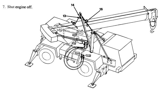
Figure 5-22 Lifting the Upperstructure
