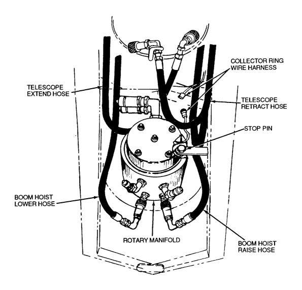
Figure 5-40 Rotary Manifold Hoses
