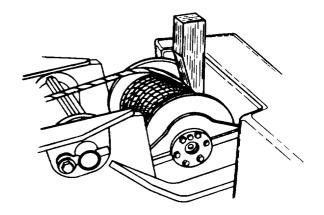
Figure 5-6 Wedge Block in Winch Drum
