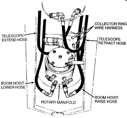
Figure 5-19 Rotary Manifold Hoses
