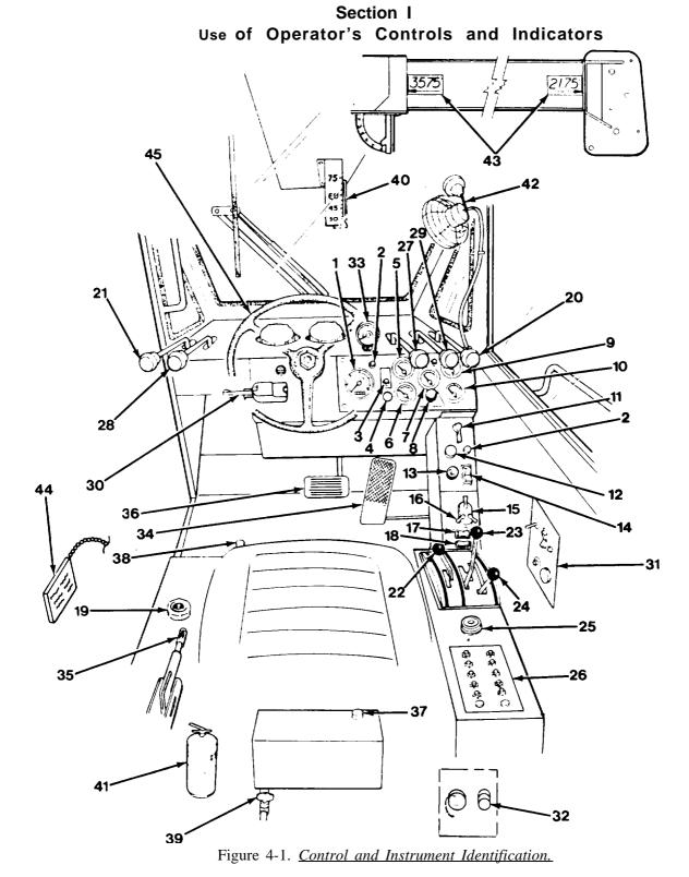
The controls and instruments are illustrated from operator's view point with the machine in travel position.
