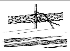
Figure 4-29. Seizing Wire Rope - Method A
