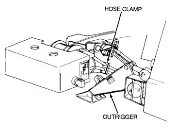
Figure 5-34 Positioning Outrigger
