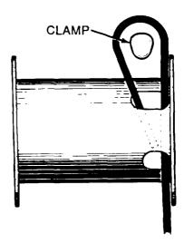
Figure 2-6. Securing Cable on Winch
