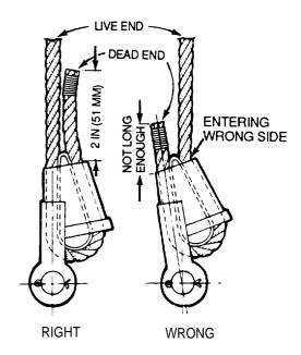
Figure 4-38. Installing the Wedge Sock et
