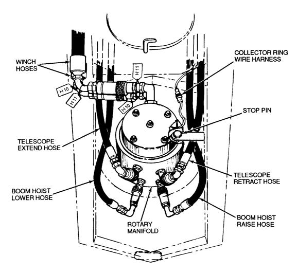
Figure 5-13 Rotary Manifold Hoses
