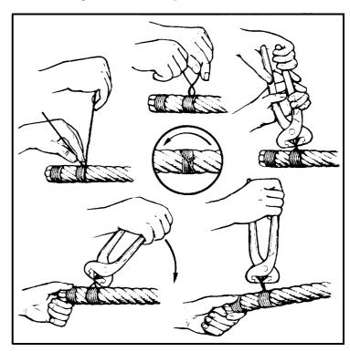
Figure 4-30. Seizing Wire Rope - Method A
