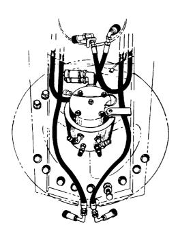
Figure 5-20 <u>Location of Boom Hoist Cylinder Hoses</u> <u>After Disconnection</u>
