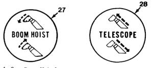
Figure 4-8 . Boom Hoist Laver Figure 4-9. Boom Telescope
