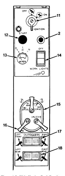
Figure 4-3. Slide Sloping Dash Panel
