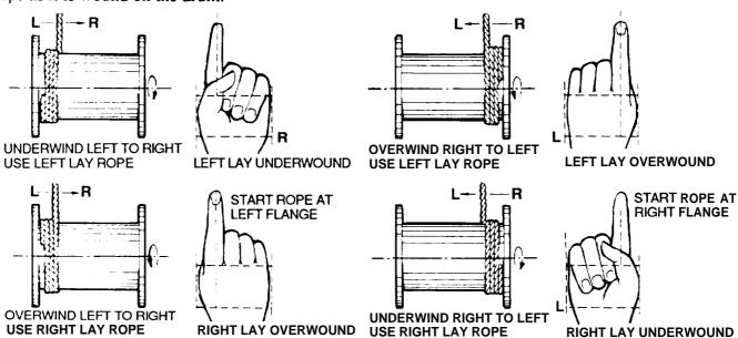
Figure 4-40 Drum Winding and Appropriate Hand Signals
