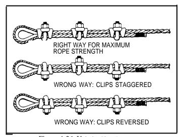
Figure 4-36. <u>U-bolt Clip Dimensions</u>
