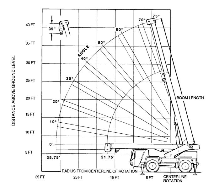
Figure 1-6. Radius from Centerline of Rotation
