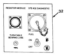
Figure 4-13. Diagnostic Connector Panel
