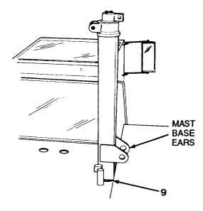
Figure 5-10. Assembling the Mast
