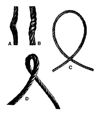
Figure 4-22. Wire Rope Kinking
