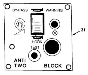
Figure 4-12. Anti-two Block Panel
