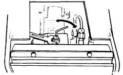
Figure 4-54. Holding Valve (Adjusting Screw)
