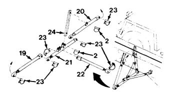
Figure 5-29 Support for Front of Boom
