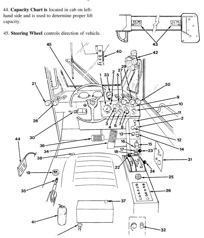
Figure 4-1. Control and Instrument Identification
