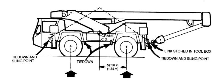
OVERALL LENGTH 342 in. (8.69 m) OVERALL HEIGHT 93 in. (2.36 m) SHIPPING CUBAGE 1767 cu. ft (50.04 cu. m) OVERALL WIDTH 96 in. (2.44 m)
