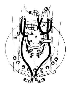
Figure 5-20 Location of Boom Hoist Cylinder Hoses
