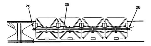
Figure 5-33 Secure Pads on Boom
