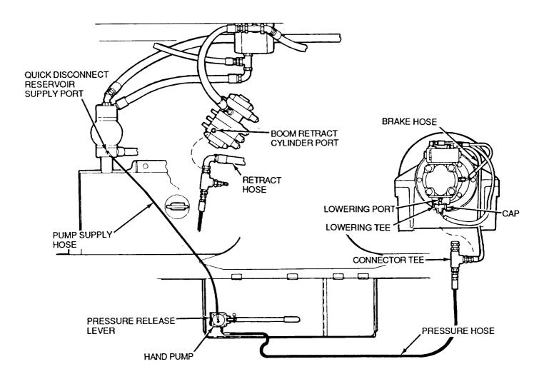
Figure 4-53. Quick Disconnect on Supply Hose
