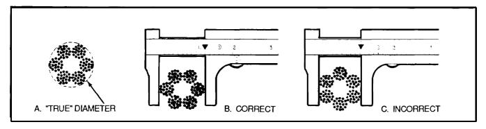
Figure 4-21. How to Measure (or caliper) a Wire Rope
