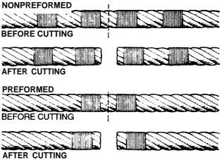
Figure 4-31. SeizinG Applied Before Cutting
