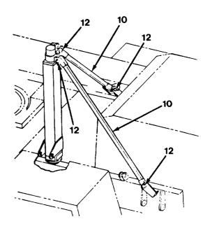
Figure 5-11A. Installing the Truss Rods
