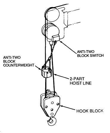
Figure **5-2.** Anti-Two Block Counterweight. Switch and Hook Block
