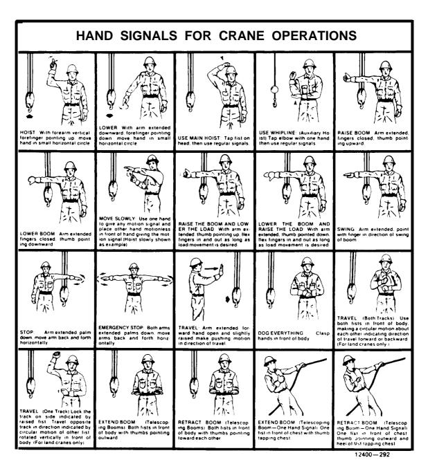
Figure 4-16. Hand Signals for Crane Operation
