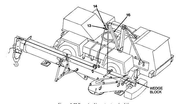
Figure 5-36 Preparing Upperstructure for Lift
