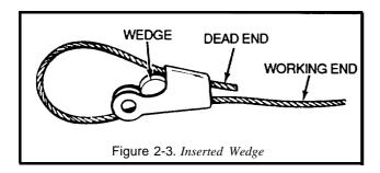
3. Seat wedge and loop just tightly enough to allow handling by attaching socket to a strong support and engaging winch to take a strain on cable.
