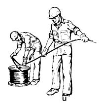
Figure 4-28. Incorrect Method of Uncoiling Wire Rope
