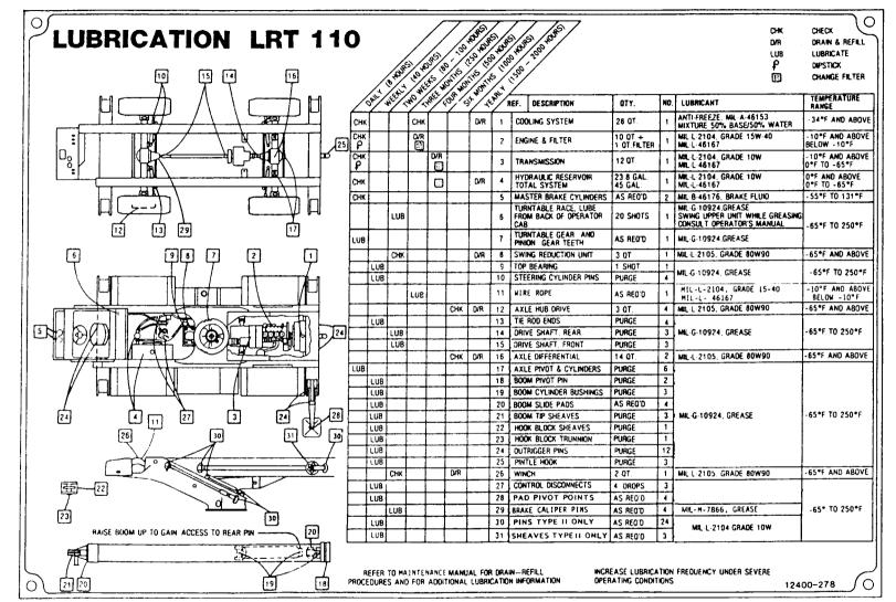
Figure B-2. Lubrication Points
