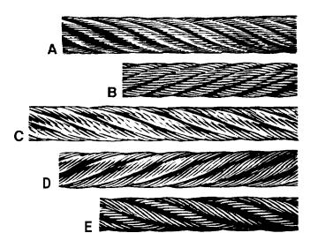
Figure 4-17. a.Right Regular Lay b. Left Regular Lay c. Right Lang Lay d. Left Lang Lay e. Right Alternate Lay.
