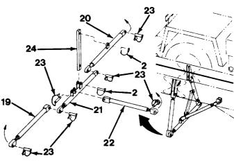
Figure 5-29 Support for Front of Boom
