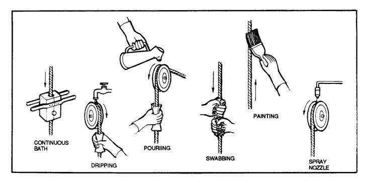
Figure B-1. Methods of Applying Lubrication
