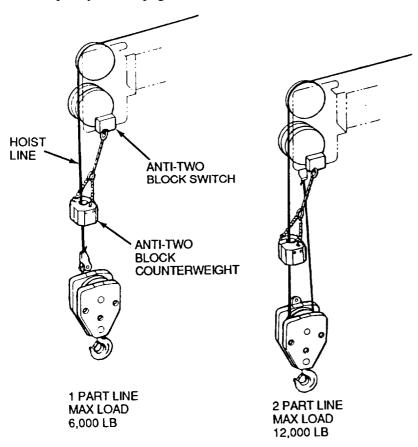
Figure 2-1. Hoist Line Reeving
