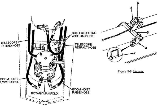
Figure 5-19 Rotary Manifold Hoses
