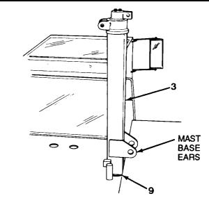
Figure 5-10. Assembling the Mast
