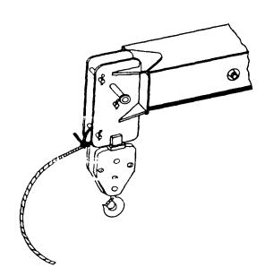
Figure 5-24 Attached Tether Rope
