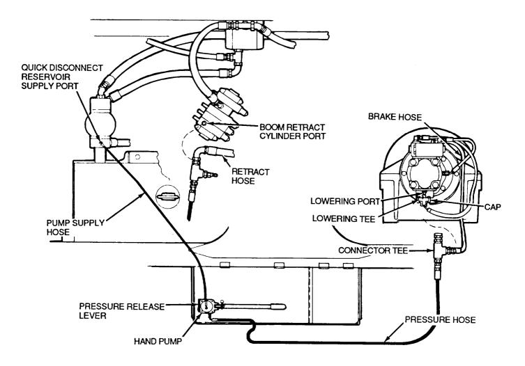
Figure 4-53. Quick Disconnect on Supply Hose
