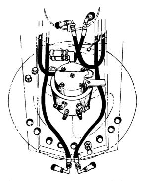
Figure 5-20 <u>Location of Boom HoistCylinder Hoses</u>
