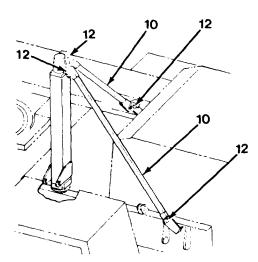
Figure 5-11A. *Installing the Truss Rods*
