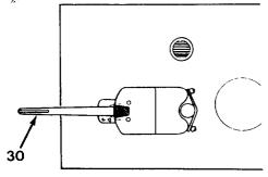
Figure 4-11. Turn Signal Lever
