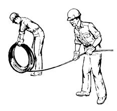
Figure 4-26. Correct Method of Uncoiling Wire Rope
