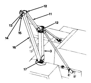
Figure 5-31 Assembling the Mast
