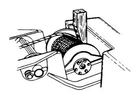
Figure 5-6. Wedge Block in Winch Drum
