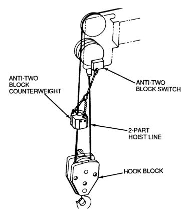
Figure 5-2. <u>Anti-Two Block Counterweight, Switch and</u> Hook Block
