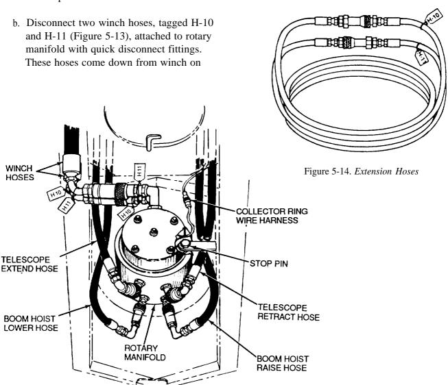
Figure 5-13. Rotary Manifold Hoses
